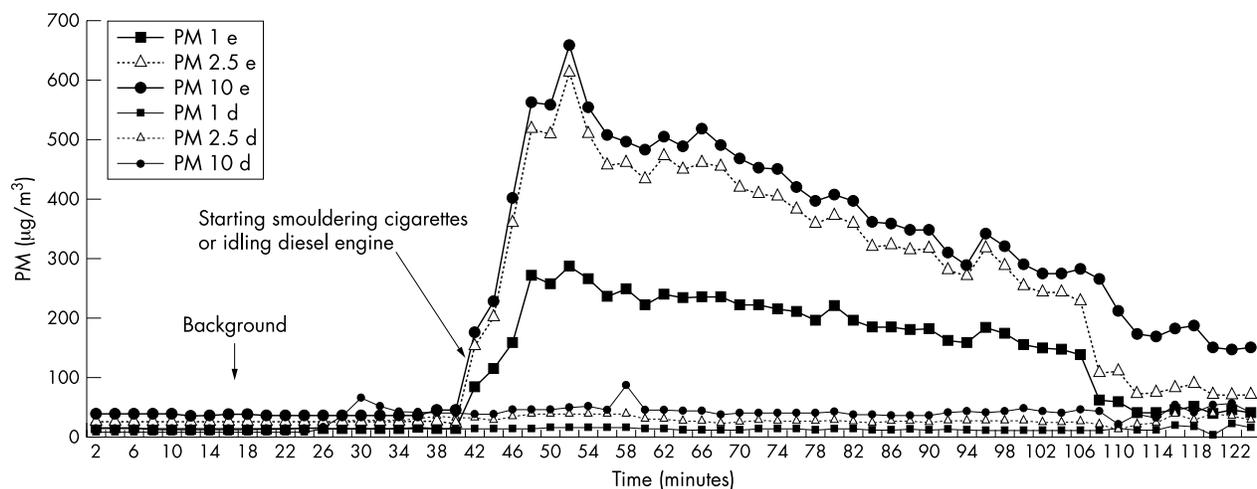
**Figure 1** Particulate matter (PM) production from environmental tobacco smoke (e) and an ecodiesel engine (d) (three smouldering cigarettes or an idling engine for 30 minutes in a 60 m<sup>3</sup> garage).
